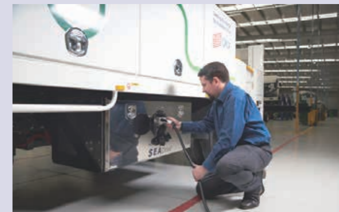
In 2020, ORIX Australia began leasing SEA Hino 917 EV carbon-free electric trucks produced by SEA Electric* 3 to a major New Zealand Group company that is in the road and airport infrastructure construction and maintenance business. The world's first electric truck, the SEA Hino 917 EV has a power system with a battery capacity of 100 kWh and a maximum range of 275 km (unloaded) on a single charge. Lessees also consider this to be a key initiative aligned with their management philosophy of providing sustainable infrastructure development.
