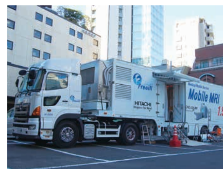
Vehicle equipped with an MRI machine
