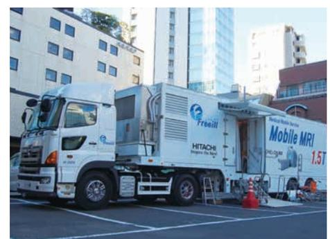
Vehicle equipped with an MRI machine
