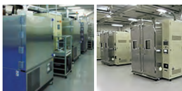
Charging and discharging testing equipment
