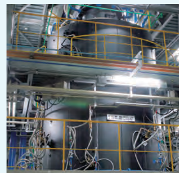
High-temperature reactor that melts waste
