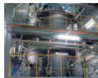
High-temperature reactor that melts waste
