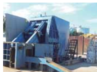
Scrap metal compactor
