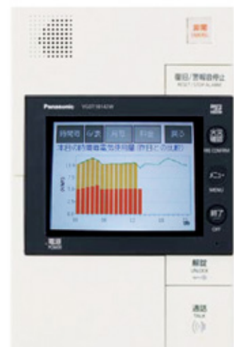
Visualization of electricity usage using intercom screen
