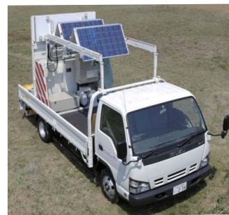
Low-emission vehicle equipped with a solar-power system
