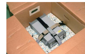
M-Cross Packaging (Hook-and-loop fasteners hold products in place, making cushioning materials unnecessary)
