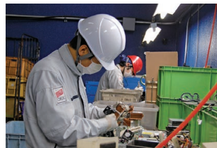
Dismantlement and sorting of OA equipment
