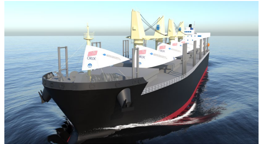
Image of the vessel with wind propulsion system installed (Image courtesy of Sumitomo Heavy Industries Marine&Engineering Co., Ltd.)
