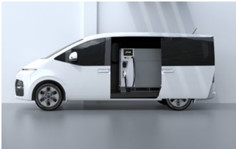
Van mounted rapid charger
