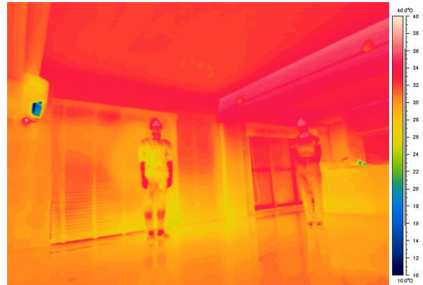
Uneven temperature environment in the unit due to insufficient thermal insulation and sunlight-shielding performance
