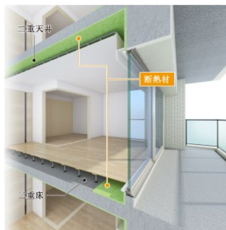
Image of high-insulation material applied to ceiling and floor
