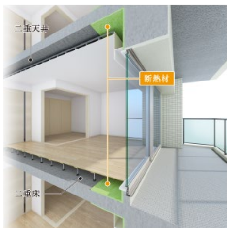
Image of high-insulation material applied to ceiling and floor
