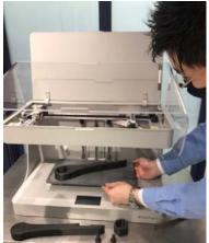
The Form 3 is a stereolithography (SLA) printer that features low-force stereolithography (LFS) technologies\*2. It is capable of creating accurate and highly detailed forms, through the use of a precise, high-power laser. SLA printers can be used with an abundance of materials in a variety of different colors and, for these reasons, are suited to shape verification in product design.
