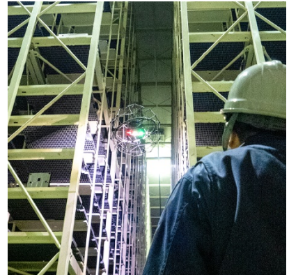
Image of indoor inspection using ELIOS
