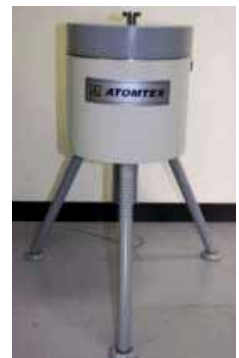
Radioactive food contamination monitor (AT1320A)
