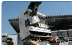
2) Waste being loaded into a crusher
