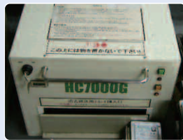
PCs with no prospects for resale, or those for which data deletion cannot be performed, have their hard disks removed and magnetically wiped.
